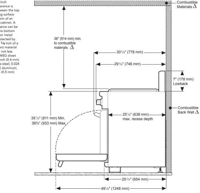
$\Delta$  As defined in the "National Fuel Gas Code" (ANSI Z223.1, Current Edition). Clearances from non-combustible materials are not part of the ANSI Z21.1 scope and are not certified by CSA. Clearances of less than 6" (152 mm) must be approved by the local codes and/or by the local authority having jurisdiction.
