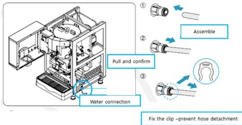
After the installation is complete, please operate the product and check whether there is leakage in the water supply and drainage parts.
