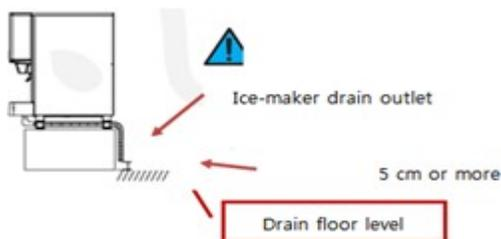
**Be careful not to bend the drainage hose during the installation and also confirm that the hose is not exposed to fire or sharpness which may result in the hose burst (This will become the cause of the PL accident and the manufacturer shall not be held responsible)**
