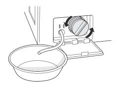
Clean the pump filter and opening.
