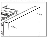
1. Before the refrigerator door handle is installed (note: the anchor bolts of the handle are in the accessory bag, and all steps should be performed at the right and left two mounting positions simultaneously.
