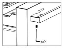
4. Wait until the handle fits perfectly with the door body, and then use a hexagonal wrench to tighten the locking screw inside the handle part.
