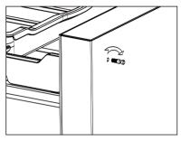
2. Screw the locating bolt into the bolt hole of the door body and secure it.
