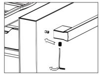
3. Loosen the locking screw inside the handle part with a hexagonal wrench first, then align the handle with the positioning bolt and insert it into the positioning bolt (note: the handle locking screw is installed facing down).
