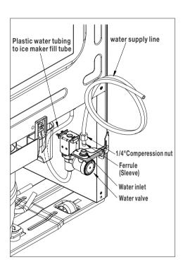
5. Turn ON water supply at shutoff valve and tighten any connections that leak.
