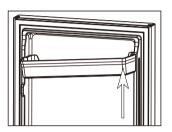
2. Maintain the first step push up at the same time, disengage the right side, and continue to take the tray off upward.
