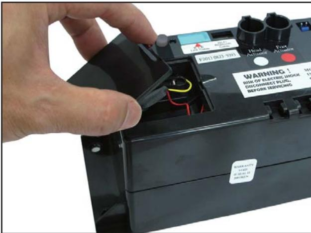
Figure 1: 9 volt batteries cover.
