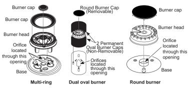
B. Using a 7 mm or 9/32" nut driver, remove the top burner orifices. These may be accessed through the burner opening in the base.
