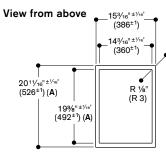
(R 5<sup>+1</sup>) A: When installing with appliance cover consider the deeper cut-out See separate notes "assembly with appliance cover" on page 113).
