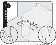
Locate anti-tip bracket hook on the floor 8-1/2" (21.6 cm) from side cabinet and 2-1/2" (6.4 cm) from rear wall when using an island trim or high shelf. \*If using an 8" (20.3 cm) backguard with spacers, add 3/4" (1.9 cm) to the 2-1/2" (6.4 cm) for a total of 3-1/4" (8.3 cm). Mark and drill 1/8" (.32 cm) holes where bracket will be located.
