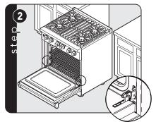
Fold latches backward until locked in place.
