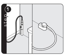
Connect gas and electrical. Before placing appliance in operation, always check for gas leaks. This must be performed by your dealer, a qualified licensed plumber, or gas service company.
