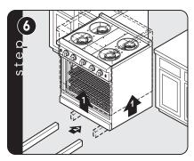
Lift unit and prop on wood blocks.
