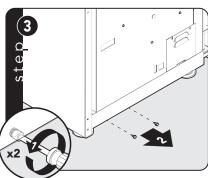
Remove two screws from back of range.
