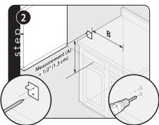
Locate anti-tip bracket on rear wall with the top left corner at measurement (A) plus 1/2" (1.3 cm) from the floor and (B - see chart) from where the right side of range (facing range) is to be located.
