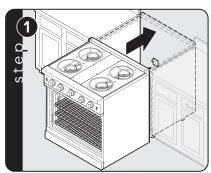
Slide range into place. Be sure wall anti-tip bracket slides into the anti-tip opening or floor anti-tip hook and bracket are engaged (depending on the one used)
