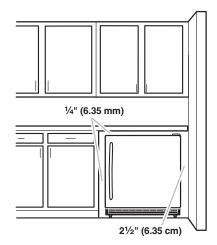
To ensure proper ventilation for your refrigerator, allow for a 1/4" (6.35 mm) space on each side and at the top. When installing your refrigerator next to a fixed wall, leave 21/2" (6.35 cm) minimum clearance on the hinge side to allow for the door to swing open.
