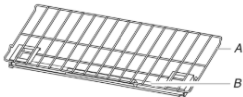
A. Steam rack B. Water reservoir
