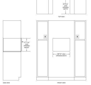
NOTE: 24" (610) and 30" (762) models require the same opening dimensions. Electrical supply must be located in adjacent cabinet within 3' (.9 m) of opening.
