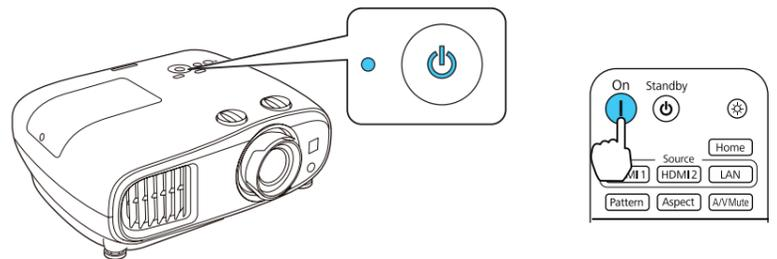
**Note:** To shut down the projector, press the power button on the projector or the **Standby** button on the remote control, then press the button again to confirm, if necessary. Wait for the projector to cool down before unplugging it.
