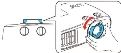
6 If your image is uneven on the sides, you can use the keystone correction feature to adjust the image. To use this feature, you must first set the lens to the center-top position using the lens shift dials.
