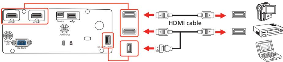
**Note:** The DC Out (2.0A) port provides power to streaming media devices.
