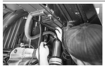
Continue to route the harness down the rear tube through the shock reservoir opening. The wire harness should follow the upper shock mounting tube.
