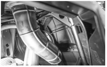
Follow the tube down towards the front of the vehicle and attach with wire tie wraps.
