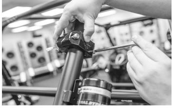
You will want to install the wake can bracket approximately 4-6 inches away from the top of the rear shock reservoir. Place the wire in the notch on the side of the clamp before tightening so the wire does not pinch.
