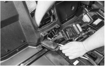
Feed both wires under the access panel and connect to RFRZ-4KD or RFRZ-PMXWH1 rear speaker harness.
