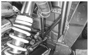
Route the harness toward the center of the vehicle toward the rear access panel.
