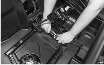
Once connected, bundle up any slack in the harnesses and wire tie wrap to hold in place.
