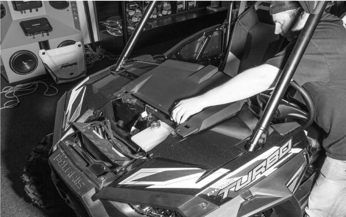
Disconnect all of the wires connectors and set aside.
