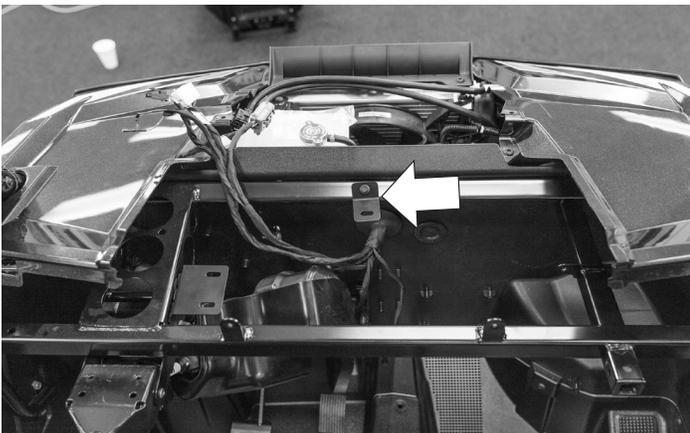
Attach the new bracket with the existing bolt that previously held the center pocket bracket.
