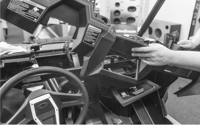
Once the bolts are removed you will need to pull the dash off of the chassis.
