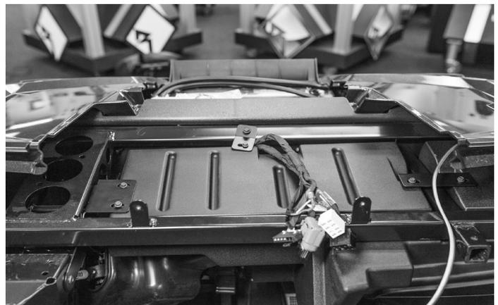
**NOTE:** The vehicle's wire harnesses that were removed from the dash top will go between the enclosure and the fire wall. There is a groove on the enclosure where the wires are to be routed.
