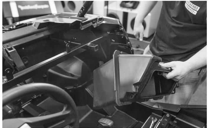
Remove the glove box from the vehicle once bolts are removed.
