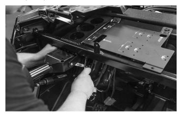
Tighten the two nuts on the steering column bracket.
