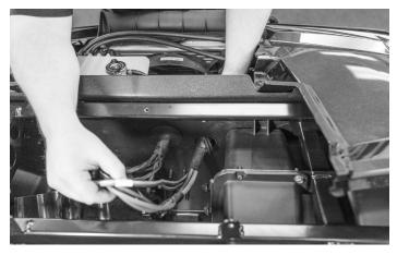
Pull the wire harness through to provide enough slack for when mounting the amplifiers.
