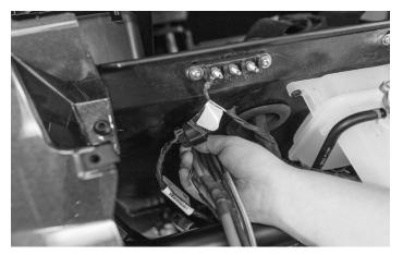
Insert the wire harness in through the opening on the fire wall and lock the grommet in place.
