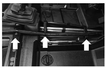
NOTE: Be careful to mount the wire harness on top of the center console supports so it will be clear of moving drive line components.
