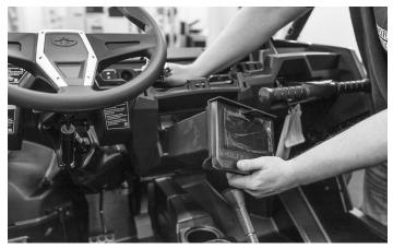
After the brace is disconnected from the center pocket, pull the pocket out of the dash.
