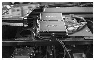
Plug in the RCA cables at this time as well. Route them in between the amplifier and the tab. Place the loose ends down toward the back of the center pocket location.
