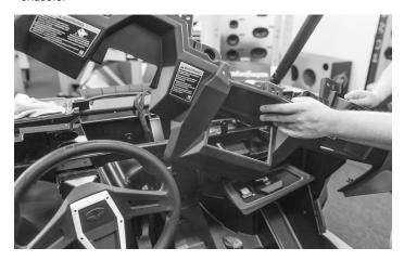
NOTE: When pulling the dash off you will notice that it still feels attached. It has several retaining clips on each side that are holding it in place. Just continue pulling toward the interior of the vehicle to release the dash from the chassis.
