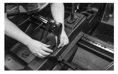
Disconnect the rubber boots on the shifter and seat belts by squeezing them inward to loosen them from the console.
