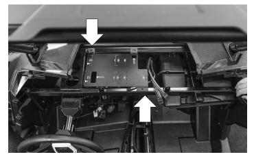
Lay the bracket on top of the dash bar and align the notches with the two bolts that were just loosened on the steering column.
