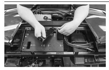
Now install the center pocket brace back into the vehicle in between the amplifier bracket and the fire wall support bar. Use the existing factory hardware.
