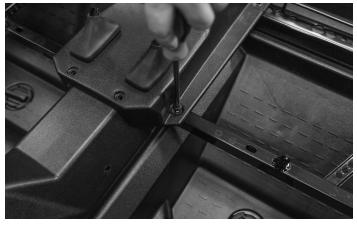
Next remove the bolts and plastic retaining clips. Use a small flat blade screwdriver to pry the plug out of the retainer so it can be removed.
