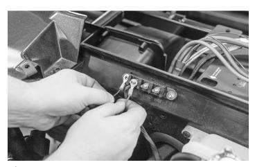
Connect the ring terminals to the factory accessory power distribution block. The power ring terminal gets connected to the ACC and the ground ring terminal gets mounted to the screw to the left.
