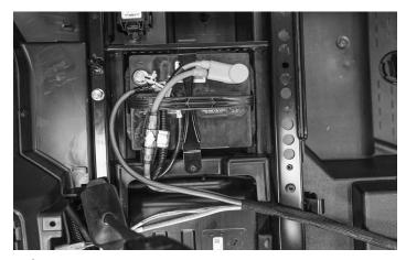
NOTE: If you have a 2 seater, the wire harness will need to be bundled up and tie wrapped. Do not cut the harness. There is enough clearance with the extra wire length.
