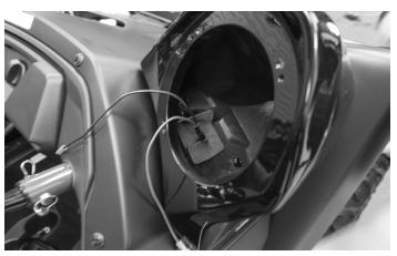
NOTE: Be sure leave adequate wire length to attach the speaker.
