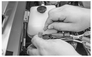
Connect the remote turn on wire to the PMX-2 harness under the hood, along with any other speaker connections.
