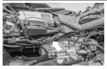
Once all connections are made at the amplifier, begin to route the harness down the passenger side of the vehicle following the main vehicle harness. Tuck the audio harness under main vehicle harness to avoid the panel bulging.
