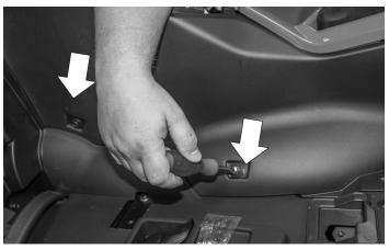
The passenger side transmission tunnel plastic panel has (3) bolts and (5) plastic rivets securing it to the chassis.
