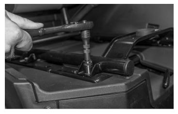
There are (4) mounting bolts holding the seat frame in place. Remove these bolts using a 12mm socket and rachet. Then, lift the seat assembly out.
