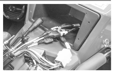
Plug the RCA's from the main harness into the back of the PMX-2 and slide radio into the center console. Secure dash kit to the center pocket once everything is connected.
