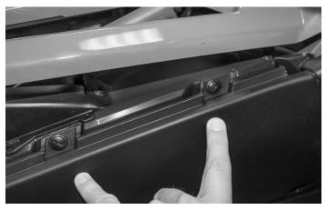
Once the plastic rivets are removed, lift up on the shifter surround plastic to expose (2) more rivets needed for the removal of the plastic side panel.
