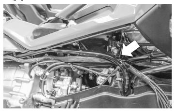
Secure the main audio harness the shifter support with the supplied zip ties.
