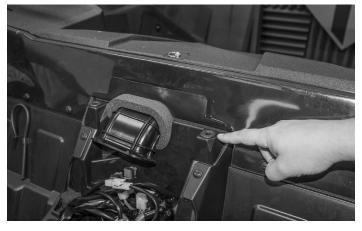
NOTE: When removing, be sure to make sure the rubber grommets are in good condition and inserted correctly. If they are not installed properly, the center console will not engage the correct way or attach securely.
