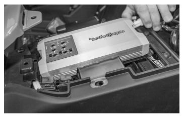
Insert the tongue end of the bracket first to capture the bracket on the plastic support panel below the shifter.
