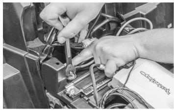
Connect the power and ground wires to the battery. NOTE: Be sure to test the system before reassembling the vehicle.
