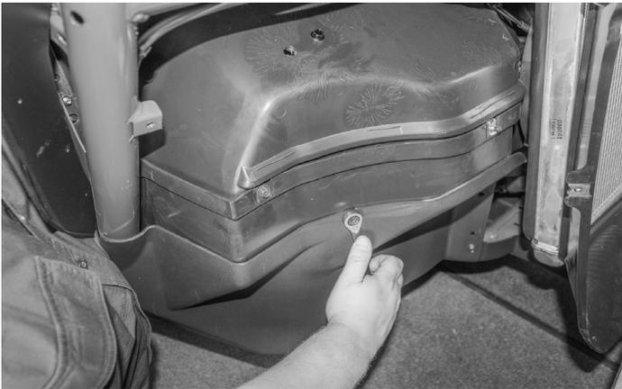
Finish securing the speaker pod in place with the (2) bolts used earlier.
