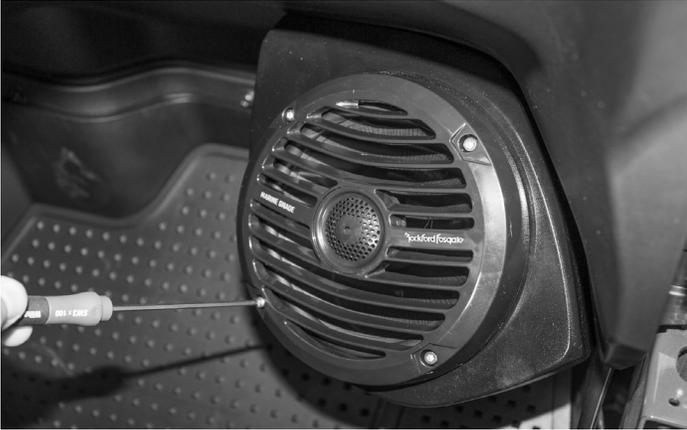
Load the speaker into the enclosure and secure using the hardware supplied with the speaker.
