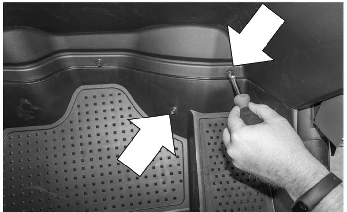
Remove the (2) bolts from the inside of the vehicle on both the passenger and driver's side.
