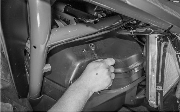
Install using the supplied bolt through the top of the enclosure. The bolt will go through the drilled 5/16" hole. Secure with the supplied nut.
