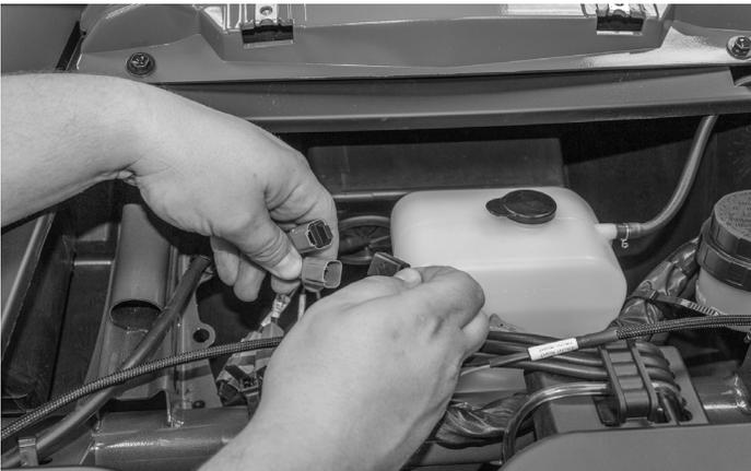
Once both speaker pods are installed and the harnesses are ran, locate the front speaker output connections in the RFXYZ-DK radio harness or the RFXYZ-K8 harness and remove the watertight plugs.
