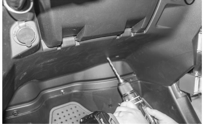
Remove the pod and drill (2) holes in the firewall using a 5/16" and 1/2" drill bit.
