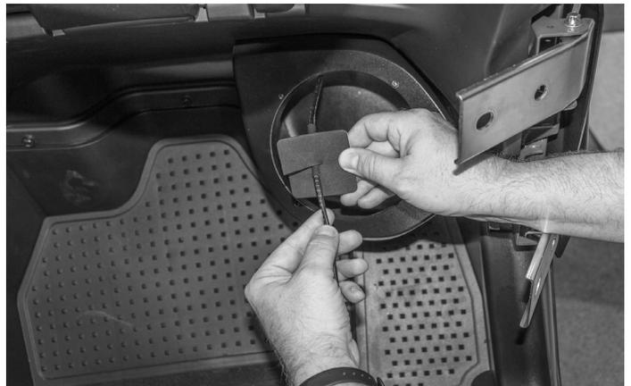
Apply the supplied foam sealing tape to the inside of the speaker enclosure to make sure you have a weather tight seal.
