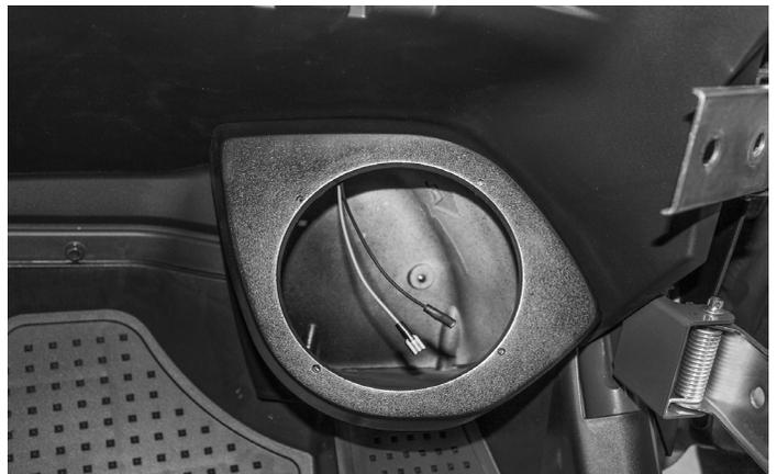
Attach the speaker wire harness connectors to the speaker terminals.
