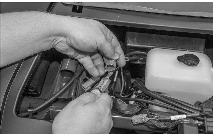
Connect the speaker harnesses to the output plugs paying attention to the left and right speaker labels.
