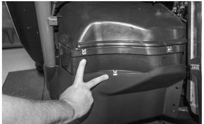
Remove the (2) spring nuts from the panels once the bolts are out of the way using a pick tool or small flat blade screwdriver.
