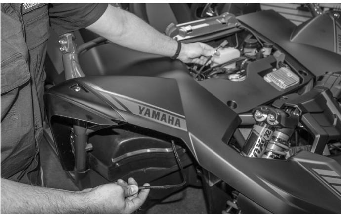
Take the speaker wire harness and run from the RFYZ-K8 or RFYZ-PMXDK harness under the hood to the holes drilled in the foot well.
