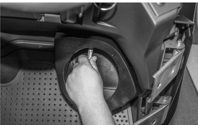
Using a marker, mark the location of the (2) holes on the top of the speaker pod for drilling.
