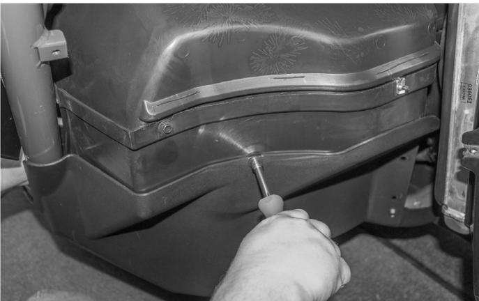
Using the (2) bolts removed from the inside of the vehicle, secure the pod in place from the wheel well side.
