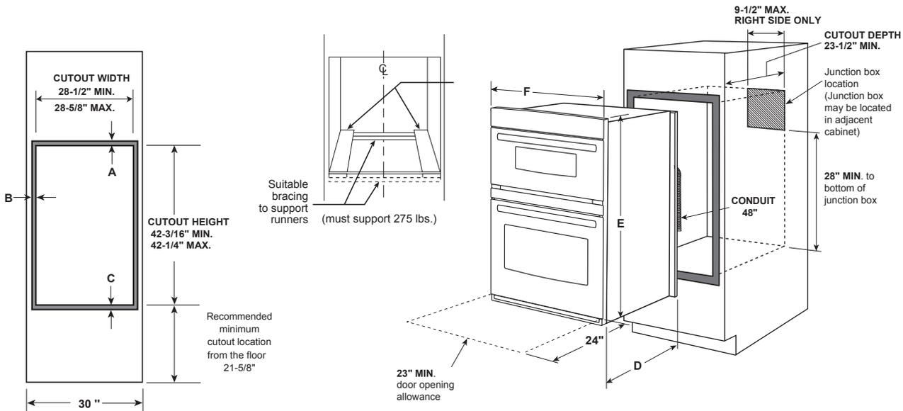
**ATTENTION INSTALLER:** All electric wall ovens must be hard-wired (direct-wired) into an approved junction box. A plug and receptacle is NOT permitted on these products.
