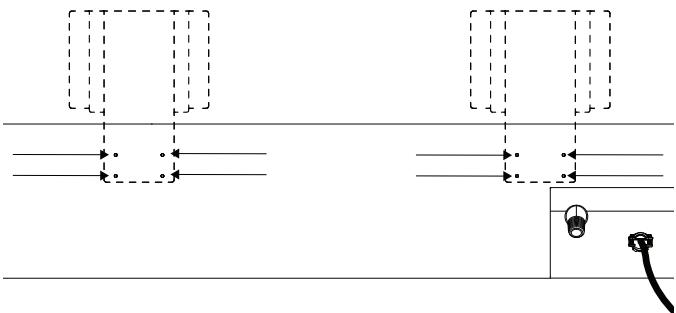
4. Secure the front of the Low Backguard to the rangetop with 2 or 3 x ½" (12.7 mm) screws.
