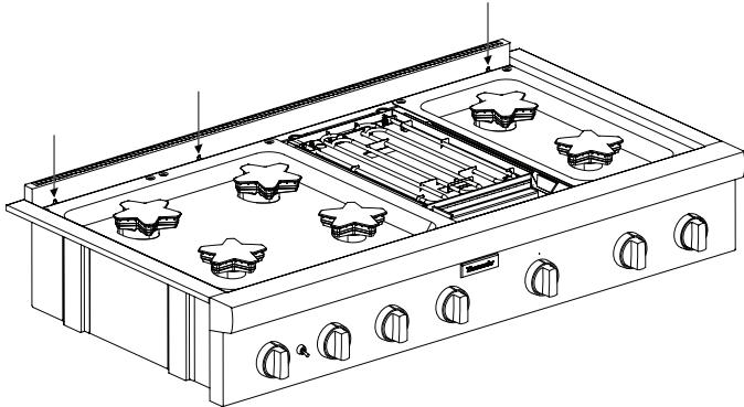
2. Slide the support brackets of the Low Backguard between the two rangetop chassis back panels.
