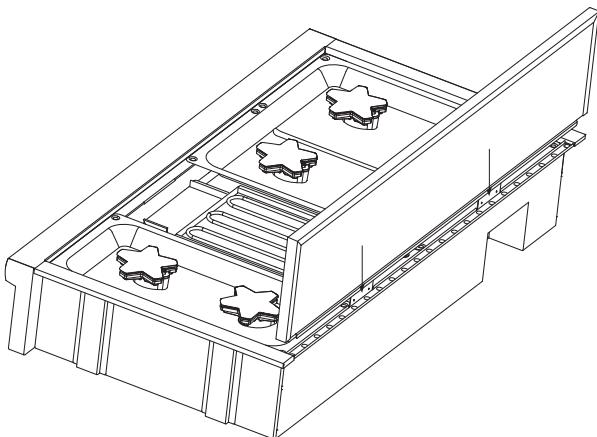
3. Secure the back with 8 x 1½" (38 mm) screws provided.
