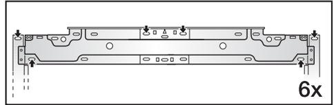
The fixing frame has several different types of holes to take account of a variety of cabinet fronts.
