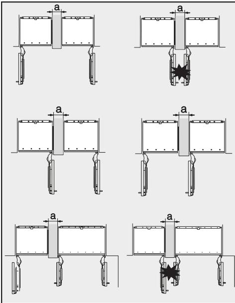
The wall **a** between the side-by-side wine conditioning unit/appliances must be **at least 5/8" (16 mm)** thick.
