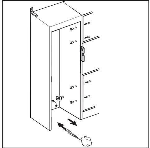
The installation niche must be carefully aligned using a level before installing the wine conditioning unit. The niche corners must be at 90° angles to each other, otherwise the cabinet door will not sit straight on all four corners.
