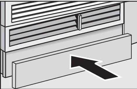
Do not cover the vents in the base. This will damage the wine conditioning unit!
