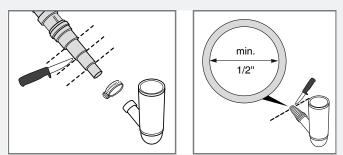
Connect the drain hose to, for example, the sink's water trap. The connection nipple must have an internal diameter of at least 1/2". The water trap must be ventilated.
