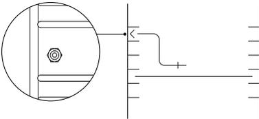
Place food in the oven and plug the probe into the socket inside the oven, on the left hand side.
