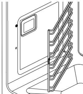
Slide the side rack forward until the rear prongs are clear of the holes.
