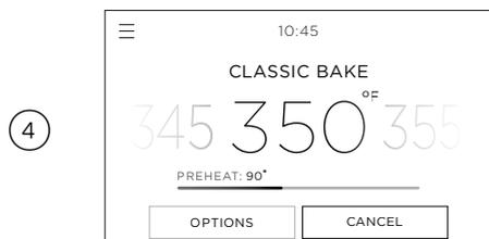
When the oven has reached the set temperature, a tone will sound, the bar will disappear and the dial\* will turn white.
