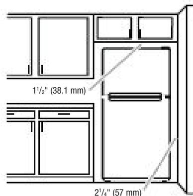
To ensure proper ventilation for your refrigerator, it is recommended to allow a 1/2" (1.27 cm) space on each side. Allow 1 1/2" (3.81 cm) of space between overhead cabinets and refrigerator top. Allow at least 1" (2.54 cm) between back of cabinet and the wall (consider the condenser as back in case is present). If your refrigerator has an ice maker, make sure you leave extra space at the back for the water line connections.
