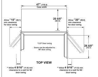
\*\*\* These refrigerators are equipped with a 3-position door stop. The factory-set 115° door swing can be adjusted to 90° if clearances to adjacent cabinets or walls is restricted. Allow a 15" minimum clearance to wall for pan removal. If the 90° door stop position is used, pan access is maintained, but pan removal is restricted. A 130° door swing option is available for standard installation only. Dimensions based on custom handle height of 2-9/16" (6.5).
