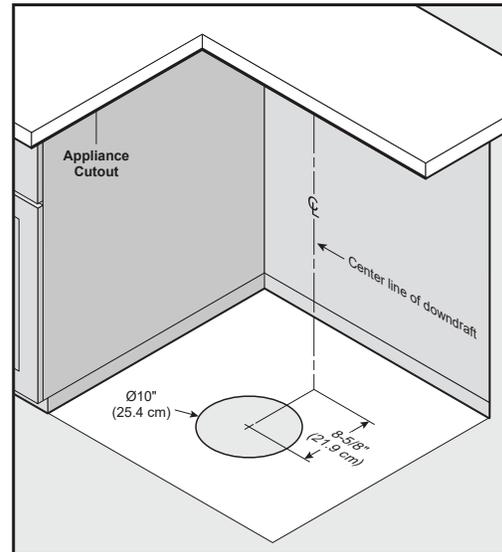
*Dimensions based off of Model 418 - 10" round elbow*
