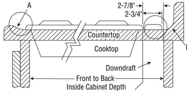
Refer to the cooktop installation instructions for dimensions of cooktop, countertop cut-out, and cabinet requirements. However, it is recommended that oversized cabinets be used for easier installation. Custom island designs need to account for deeper cabinets - especially when installed with a range in front of the downdraft or when mounting the blower behind the downdraft. You must also plan for an access door.
