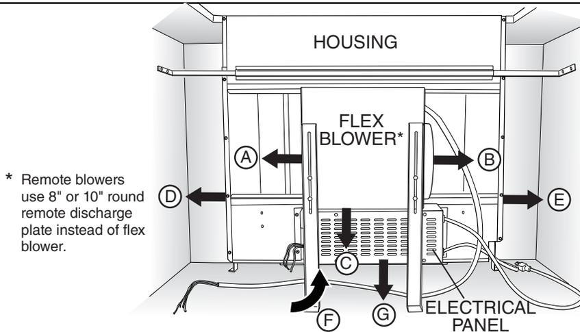
The downdraft blower system is designed for use with 8" round ductwork using a Flex Blower or 10" round ductwork using a remote blower. (Purchase blowers separately.) Seven (7) different discharge connections are available - with side-to-side adjustment for accurate alignment of ductwork:
