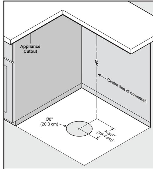
*Dimensions based off of Model 432 - 8" round elbow*
