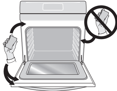
Figure 34: Clean around the oven door gasket
