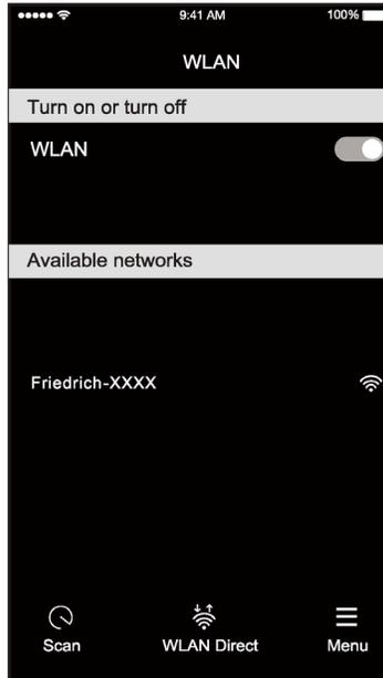
8. After connecting to " Friedrich-XXXX " network using the AC unit's Wi-Fi adapter, return to the FriedrichGo App to resume setup.
