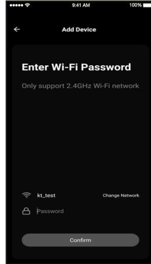
3. After connecting to the wireless network, The FriedrichGo App software will automatically try to pair the AC unit. The AC unit's LED screen may display "PP" or "SA", indicating it is searching for the network signal. This may take 10-15 seconds to connect the AC to the network.
