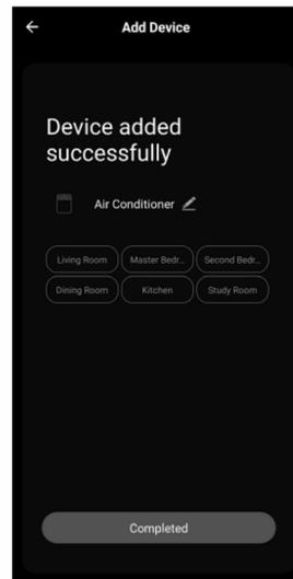
NOTE: Once your unit cycles on and off after using the AC unit's Wi-Fi adapter to connect, the AC unit will automatically pair with the network your phone is connected to.
