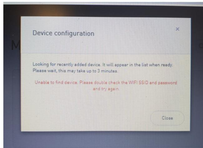
This means the consumer has entered the wrong WI-FI network name (SSID) or password.
