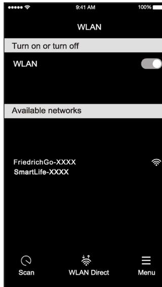
8. After connecting to Friedrich-XXXX or SmartLife-XXXX network using the AC unit's Wi-Fi adapter, return to the FriedrichGo App to resume setup.
