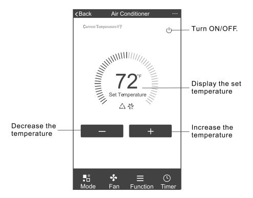
2. Adjusting settings for operation mode, Fan, Dry, Heat or Cool. Tap the "Mode" button and choose the mode.
