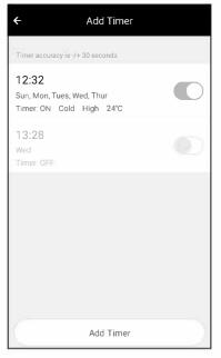
Click "ON" or "OFF" button to set Timer ON or Timer OFF. You can set the: Hour, Minute, Operate Mode, Operate Fan Speed, Operate Temperature. You can also set a weekly timer.
