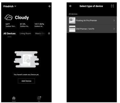
Connecting your AC to a wireless network can be completed using AP (Access Point) Mode. (Reminder-The FriedrichGo App only works on 2.4 GHZ networks)
