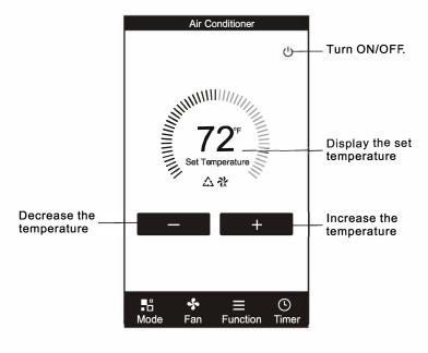
2. You can adjust the settings for the different operating mode you want to use. Click the "Mode" button and choose the mode you would like to change. Note: Some units also have a heat function. The Heat mode on the App will not be functional or change any settings on AC units that are cool only.
