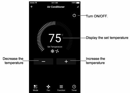
2. You can adjust the settings for the operating mode you want to use: Cool, Heat, Dry, Fan. Click the "Mode" button and choose the mode you would like to change. Note: Some units also have a heat function. The Heat mode on the App will not be functional or change any settings on AC units that are cool only.
