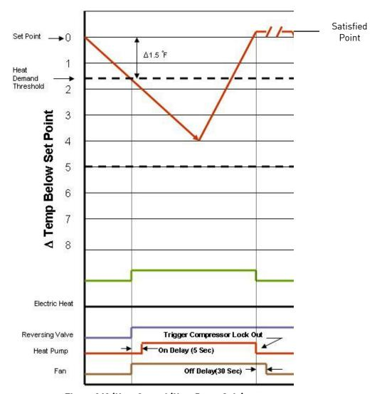
Figure 343 (Heat Control (Heat Pump Only)
