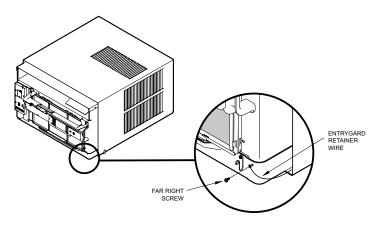
Figure 501 (Chassis Removal and Installation)
