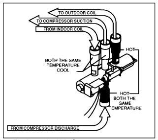
Figure 703 (Checking The Reversing Valve)
