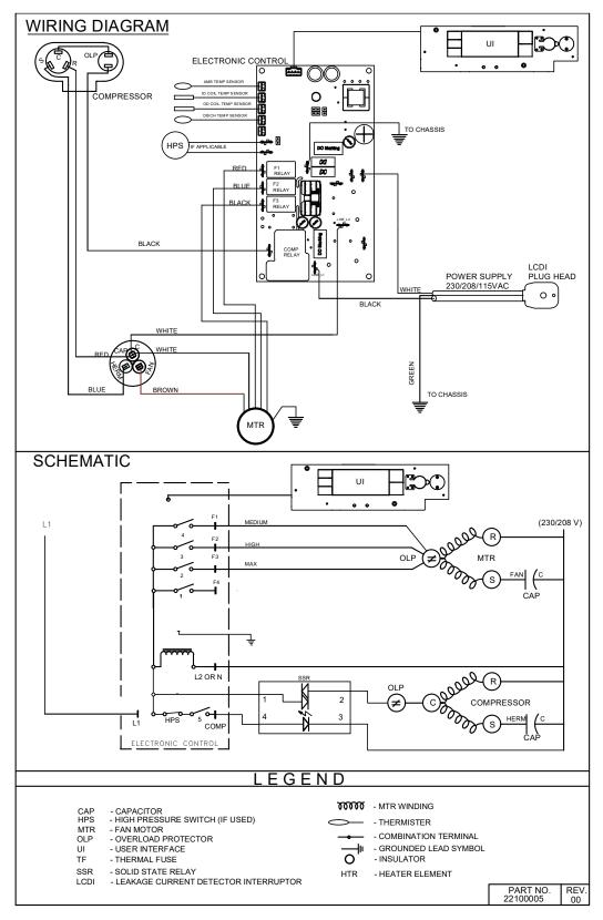
Figure 803.1 (Wiring Diagrams KCL28A30A-E)
