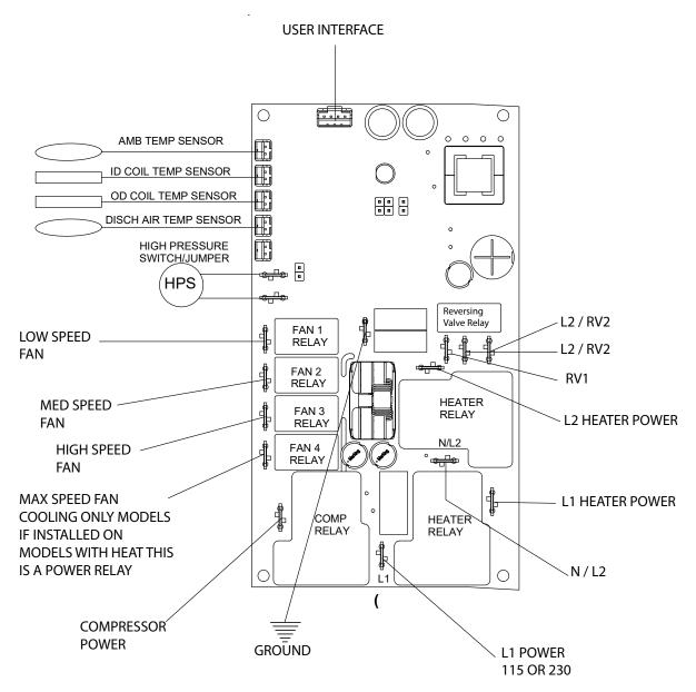
Figure 712 (Electronic Control Board Identification)
