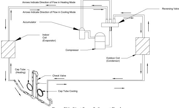
Figure 701a (Heat Pump Refigerant Flow)
