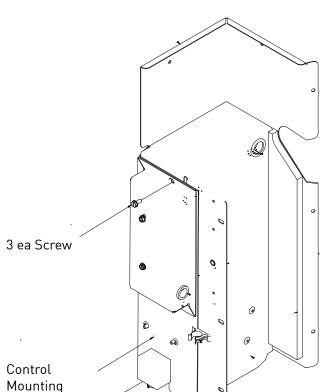
Figure 710 Access to SSR, Capacitor, PTCR
