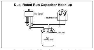
Figure 707 Dual Rated Capacitor Hook-Up
