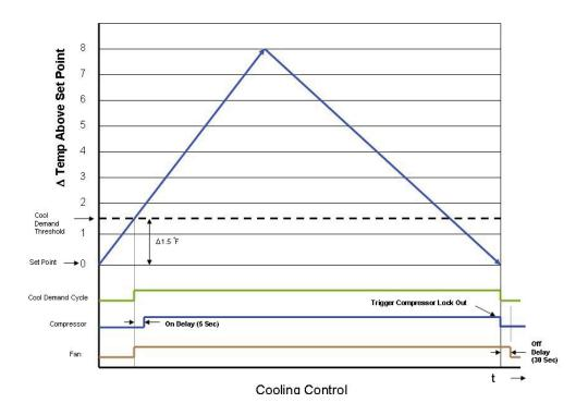
Figure 342 (Cooling Control)
