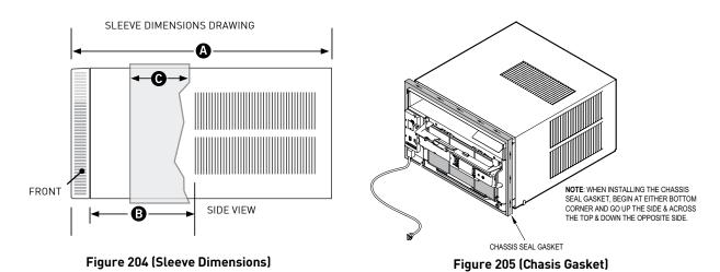
Improper installation of chasis seal gasket can cause performance problems and excessive noise or vibration. If chasis seal damage is worn, damaged, or missing, install new gasket.
