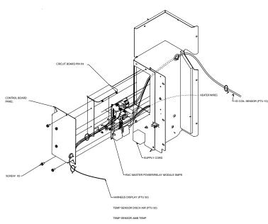
Figure 713 (Electronic Control Board Replacement)
