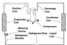
The particular system design determines at exactly what point (in the evaporator) the change of state (i.e. liquid to a gas) takes place. In all cases, however, the refrigerant must be totally evaporated (changed) to a gas before leaving the evaporator coil.
