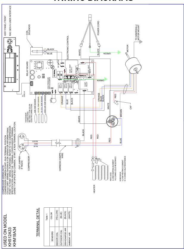
Figure 809 (Wiring Diagrams)
