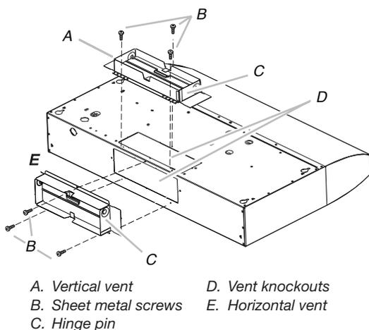
**NOTE:** If the wall cap is directly behind the vent connector, the dampers in the connector and wall cap must not interfere with each other. Remove the vent connector damper if they interfere.
