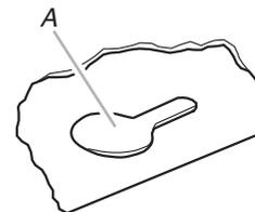
3. Use 1/8" (3 mm) drill bit and drill 4 pilot holes as shown.
