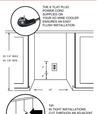
CABINET WALL TO REACH AN OUTLET INSTALLED THERE
