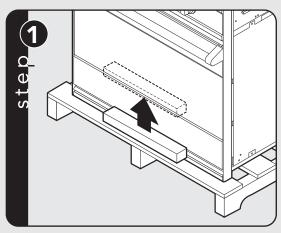
Remove wooden brace on front of pallet.
