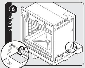
Unscrew pallet screws from side of oven.
