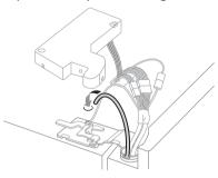
Hold the water supply connection and gently push in the collet 4 to connect the water supply line as shown. Insert the tube at least 5/8 inch (15 mm) into the connector. Insert the clip on the joint to fasten the tube in place.
