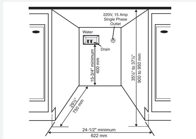
If the drain outlet is higher than 24"(610 mm), the connections will need to be recessed.
