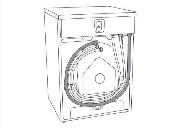
Drain hose can also be connected directly to the washbasin drain via a siphon. In this case, the hose, too, should be 24" to 36" mm above the floor. Internal hose diameter should be at least 18 mm. See figure.
