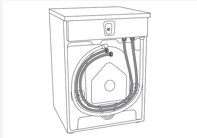
The water intake hose has to be fastened firmly enough for the hose to have a good seal. After connecting the hose, the seal must be checked for any leaks.
