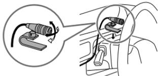
Secure using cord clamps (not supplied) if necessary.
