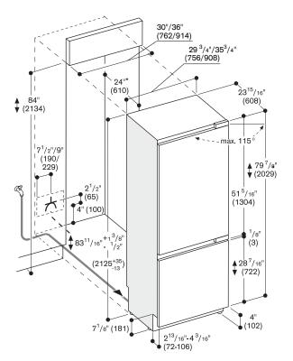
The door face dimensions are designed for a maximum gap of 1/e" (3 mm). \* For a flush-mounted appearance, the minimum cut-out depth must be 25". See more details on pages 223 and 225
