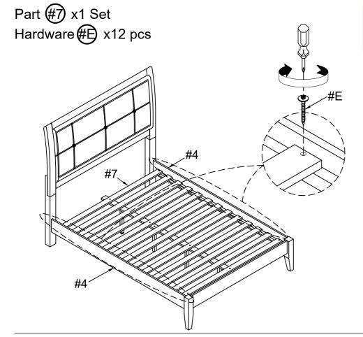
Align slats (#7) to the side rails (#4), then secure by using screws (#E).
