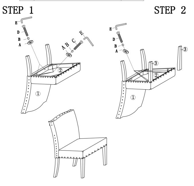
Do not fully tighten screws until fully assembled
