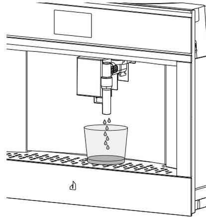
6. The coffee system will deliver fresh water from the spout then turns off automatically. The coffee system is now ready for normal use.
