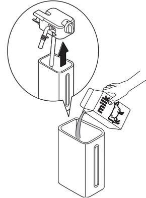
2. Fill the container with approximately 1/2 cup (100 mL) of milk for each cappuccino you want to make. Do not fill above the MAX line on the milk container. For a denser or more even froth, use cold skim or partially skim milk.
