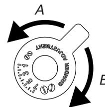
A. Counterclockwise for finer grind
