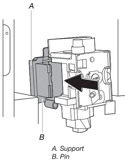
**NOTE:** If you are having difficulty replacing the infuser, compress the moving parts from both the top and bottom as shown in the following illustration before reinserting it.
