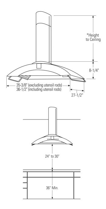
The exact installation height is determined by the ceiling height and duct cover trim strips provided with the hood. For optimum performance, the hood must be installed 24" min. and 30" max. above the cooking surface.
