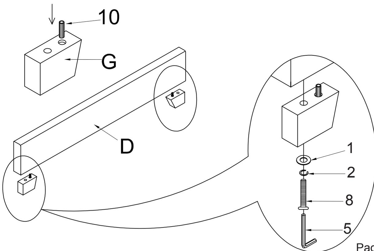
**Step 3.** Add Spring Washer (Part 2), then Flat Washer (Part 1) to Bolt (Part 9). Insert bolts into the metal bracket on the headboard legs. Do not tighten completely. Repeat this step adding bolts to the left and right sides of the footboard.
