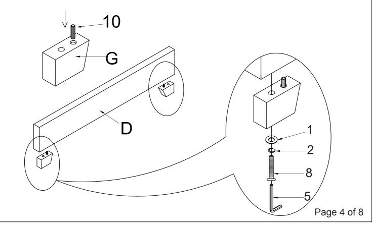
Step 3. Add Spring Washer (Part 2), then Flat Washer (Part 1) to Bolt (Part 9). Insert bolts into the metal bracket on the headboard legs. Do not tighten completely. Repeat this step adding bolts to the left and right sides of the footboard.
