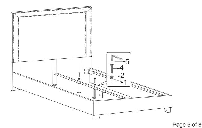
Step 7. Add Flat Washer (Part 1) to Bolt (Part 11). Attach Flat Slats (Part H) as shown using Wing Nuts (Part 12) and Allen Key (Part 13). Tighten completely.
