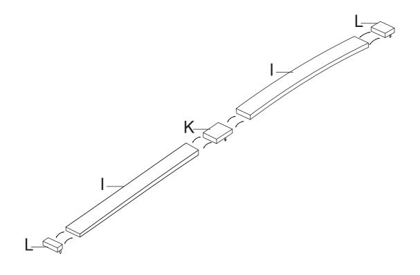
Step 9. Attach the Curved Slats pressing the Center Plastic Connectors and End Caps firmly into place.
