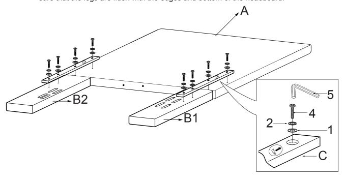
Step 2. Align bed frame with pre-drilled holes of headboard legs. Add Flat Washer (Part 1) to Bolt (Part 3). Insert bolts through the headboard legs. Add Flat Washer (Part 1) then Spring Washer (Part 2) and Nut (Part 7) and tighten using Allen Key (Part 8) and Wrench (Part 6).
