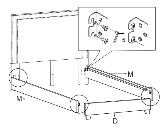
Step 5. Add Spring Washer (Part 2), then Flat Washer (Part 1) to Bolts (Parts 4 & 9). Using the Allen Key (Part 5), attach the Center Rail (Part J) to the Headboard Support Leg (Part E) and Footboard as shown. Tighten completely.
