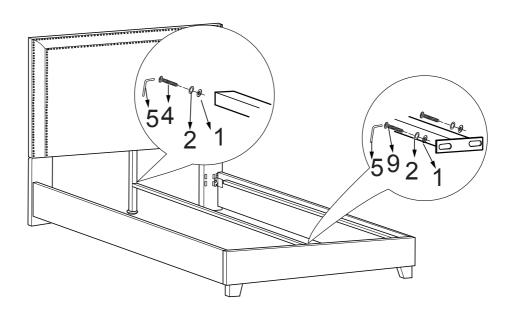
Step 6. Add Spring Washer (Part 2), then Flat Washer (Part 1) to Bolt (Part 5). Attach Center Rail Support Legs (Part F) as shown. Tighten completely.
