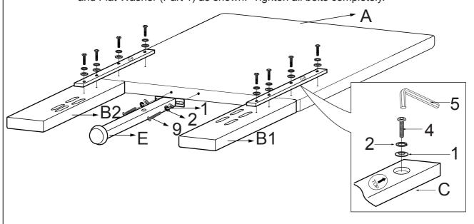
Step 2. Insert Wood Dowel (Part 10) into Wood Leg (Part G). Add Spring Washer (Part 2), and Flat Washer (Part 1) to Bolt (Part 8). Use Allen Key to attach the legs to the footboard.
