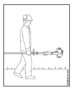
It may be carried only in a horizontal position. Grip the shaft in a manner that the machine is balanced horizontally. Keep the hot muffler away from your body and the cutting attachment behind you.
