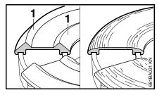
Do not continue using the mowing head if the raised moldings (1) on the base are missing or worn – see right illustration above. The mowing head may otherwise shatter and flying objects could result in injury to the operator or bystanders. Install a new mowing head.
