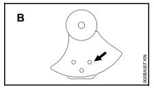
Arrows on the deflector (A) and limit stop (B) (as seen from the underside) show the correct direction of rotation of the cutting attachment. When viewed from above, however, the cutting attachment rotates counterclockwise.
