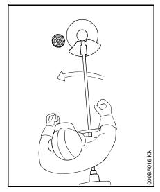
Circular saw blades are suitable for thinning brush and cutting small trees up to a diameter of 4 cm (1 1/2 in.). Do not attempt to cut trees with larger diameters, since the blade may catch or jerk the trimmer / brushcutter forward. This may cause damage to the blade or loss of control of the power tool and result in serious injury. Use a chain saw for such work.
