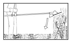
To cut wild growth and scrub, lower the rotating brush knife down onto the growth to achieve a chopping effect but keep the tool below waist height at all times.
