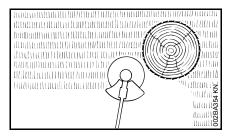
Mowing heads are to be used only on trimmers / brushcutters equipped with a line-limiting blade in the deflector in order to keep the line at the proper length (see "Main Parts" chapter in your instruction manual).
