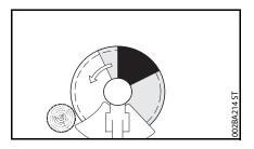
Before starting the cut, accelerate the engine up to full throttle. Perform cut with uniform pressure. STIHL recommends that the circular saw blade be applied to the right of the tree, using the non-shaded area of the blade, as shown in the illustration above.
