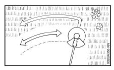
All kinds of grass and weeds can be easily cut with the grass cutting blade. The power tool is swept in an arc similar to a scythe.
