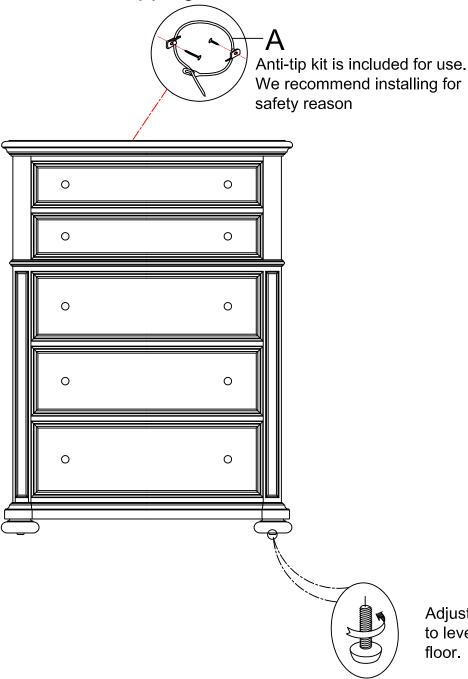
Adjust Leveler if needed to level case on uneven floor.
