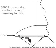
For proper operation, make sure the filters are securely seated into the channels.
