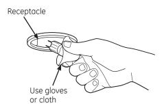
**NOTE:** Do not touch the new halogen bulb with bare fingers. Skin oils can cause early-life bulb failure.
