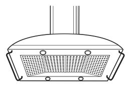
On some models, the lights arelocated on the front and back, on the underside of the hood.
