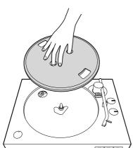
**5** Turn the platter upside down and remove the drive belt.
