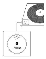
**3** Turn on the pairing mode for the playback device that supports BLUETOOTH wireless technology, to which you want to connect.
