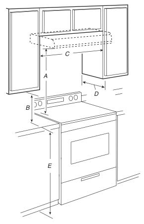
A. 18" (45.7 cm) minimum distance from electric cooking surface. 24" (61.0 cm) minimum distance from gas cooking surface. 30" (76.2 cm) suggested maximum above the cooking surface.
