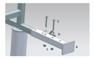
Hand tighten the Frame Bolt (C) and Locking Nut (F) in place using a flat head screwdriver and a crescent wrench.
