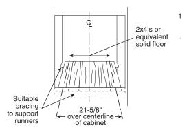
(Platform must be able to support cabinet load, weight of oven, and additional oven loads)
