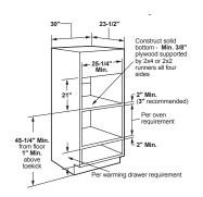
**NOTE:** Additional clearances between the cutouts may be required. Check to be sure the oven supports above the Warming Drawer location do not obstruct the required interior depth and height. See Warming Drawer installation instructions for details.
